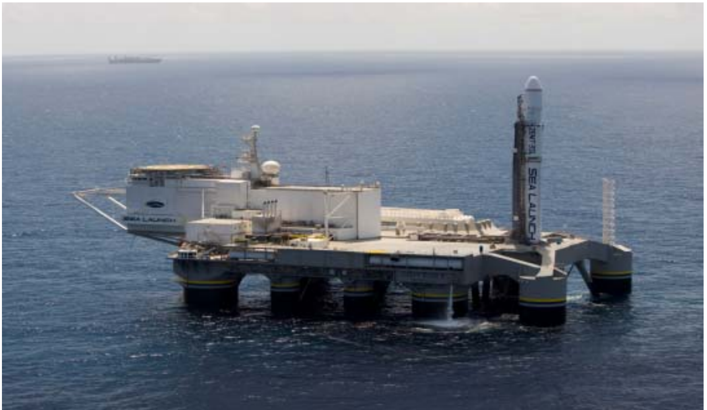
The Sea Launch vessels in launch position on the Equator, during countdown. The launch platform, one of the world's largest semi-submersible vessels, is ballasted about 65 feet for stability. The Sea Launch Commander is nearly four miles uprange, accommodating the Launch Control Center as well as remotely controlled marine operations for the platform. All personnel evacuate the platform before fueling operations are initiated. (Source: Sea Launch)
