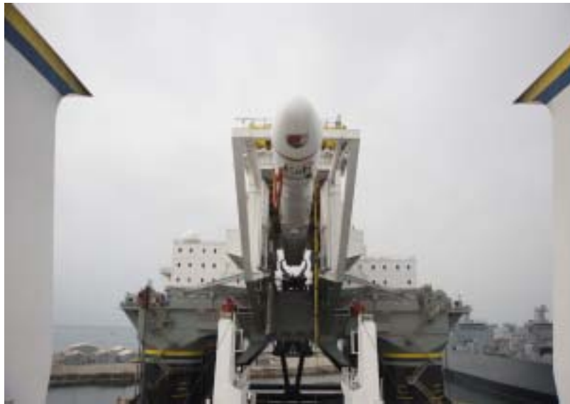
The Zenit-3SL vehicle is assembled on the Sea Launch Commander and then transferred to the Odyssey Launch Platform. This image was made from the stern of the ship, positioned directly in front of the platform during the transfer operations. The rocket is rolled onto the ship's stern ramp and then lifted 200 feet to the fore end of the hangar. Heavy cranes do the lifting and then move the rocket into the hangar, where the rocket rests on the transporter erector. (Source: Sea Launch)
