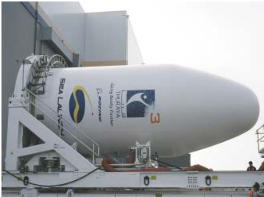
The Payload Assembly for the Thuraya-3 mission is moved out of the Payload Processing Facility onto a transporter that takes it to assembly with a Zenit-3SL vehicle, on the Sea Launch Commander. (Source: Sea Launch)
