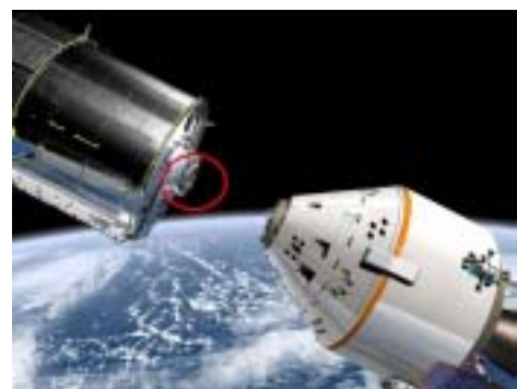
Figure 3: The Soft Capture Mechanism will be installed on the back end of Hubble during SM4 to effect soft capture by an Orion-type vehicle in the future for either de-orbit or emergency repair capability. It is circled in red for ease of identification. (Source: HST Development Office, NASA)
