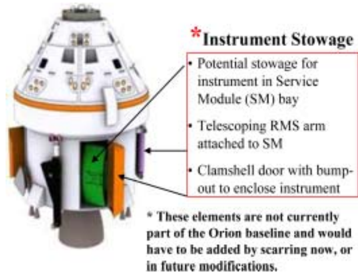
Figure 5. Instrument Stowage, a telescoping arm, and a modified door are not currently a part of the Orion baseline (Source: HST Development Office, NASA)
