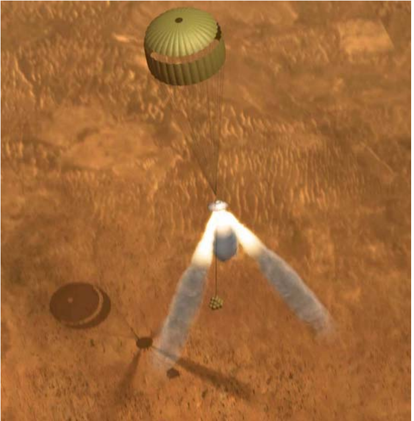
This artist's conception depicts the Mars Exploration Rover's landing sequence during the last few seconds of the spacecraft's journey. Approximately thirty to fifty feet above the Martian surface, retro-rockets are fired to slow the parachuting, airbag-padded rovers. (Source: NASA/JPL-Caltech)
