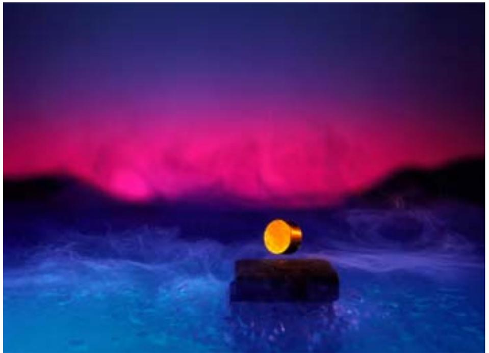
*High temperature ceramic superconductors, like the one pictured above, are made from a material that has only very low alternating-current resistance and thus dissipate less power. The magnetic forces between ceramic superconductor and magnet allow the magnet to float above the superconductor. (Source: Pacific Northwest National Laboratory)*
