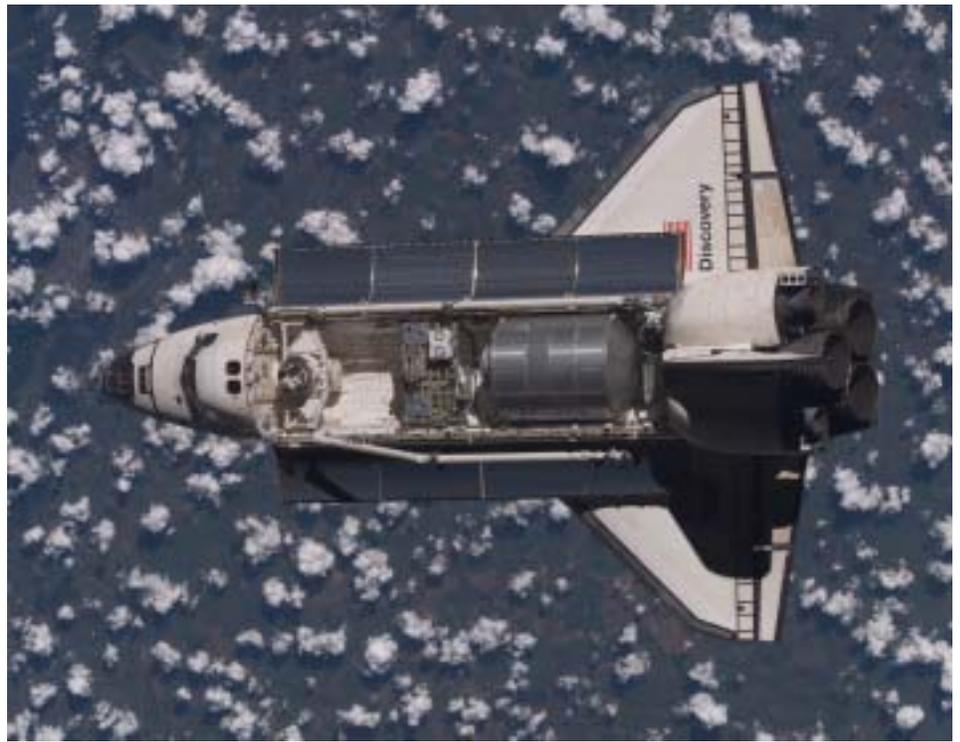
One of a series of photographs showing the Space Shuttle Discovery as taken from aboard the International Space Station during rendezvous and docking operations. The Italian-built Raffaello Multi-Purpose Logistics Module (MPLM) is in the shuttle's cargo bay. Earth, dotted with popcorn-like clouds, provides the backdrop for this image. (Source: NASA)
