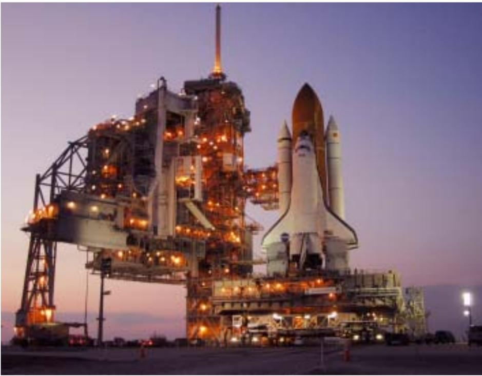
*Amid the glow of lights from the fixed and rotating service structures, Space Shuttle Discovery rests on the hardstand of Launch Pad 39B at NASA's Kennedy Space Center after completing the 4.2-mile journey from the Vehicle Assembly Building in preparation for STS-121. As the sun begins to set on the shuttle program, the challenge is to maintain the high levels of excellence needed to safely fly out the program while capturing important lessons learned for future programs. (Source: NASA)*
