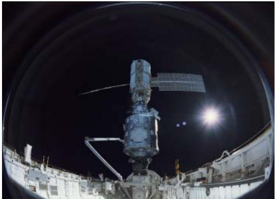
In December 1998, the crew of STS-88 began construction of the International Space Station by joining the US built Unity module to the Russian built Zarya module. (Source: NASA)
