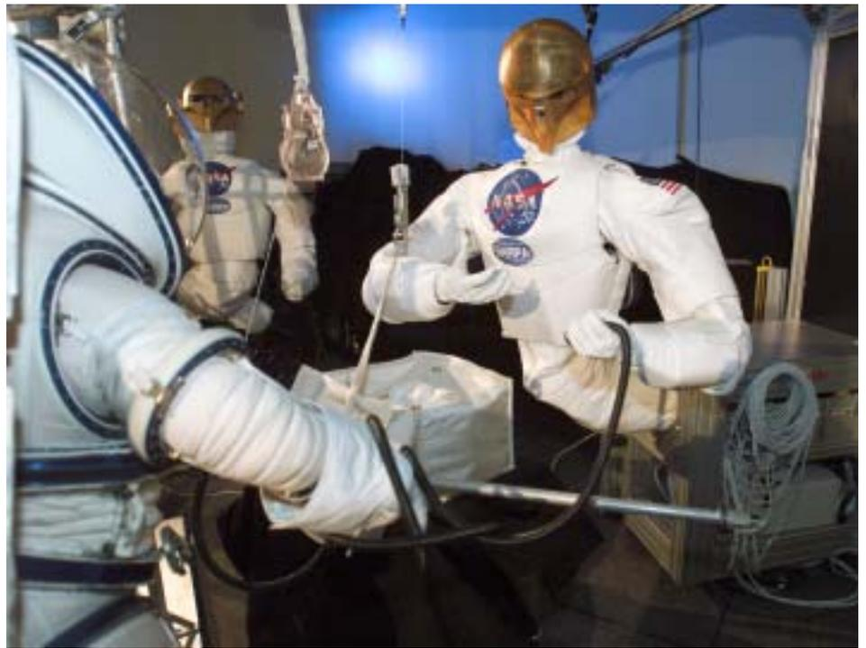
*NASA engineers at Johnson Space Center are developing Robonaut, a sophisticated humanoid robot, to assist astronauts in complex future extravehicular activities. In this photograph, one Robonaut (right) assembles an aluminum truss structure with astronaut Nancy J. Currie (left) in a demonstration scenario. A second Robonaut is visible in the background. (Source: NASA)*
