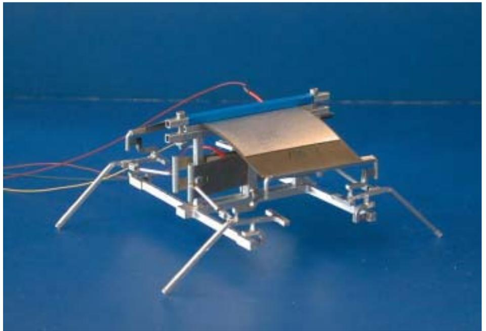
*In research funded by the Defense Advanced Projects Research Agency that could be adapted for space exploration, this mobile robot consists of a lightly damped skeletal structure that moves when vibrationally excited at the appropriate resonance. This approach allows for extremely high movement efficiency, which results in minimal power consumption and long-range mission capability. (Source: Center for Intelligent Mechatronics).*
