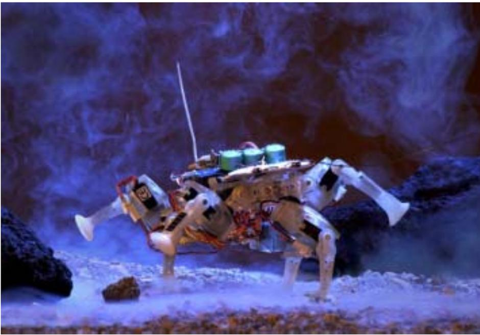
*Engineers at the Jet Propulsion Laboratory develop small robots capable of accomplishing a variety of tasks in environments that prove challenging for human exploration. The design of Spiderbot, seen here, mimics much of nature's design of the spiders we see here on Earth. Spiderbot can traverse very rugged terrain while carrying many data sensors. (Source: NASA/Jet Propulsion Laboratory)*
