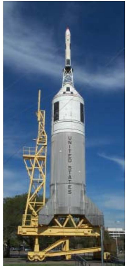
*The Little Joe II solid rocket booster, shown here, proved effective in testing boilerplate versions of the Apollo command module launch escape system before actual crewed flights. A similar launch vehicle using existing hardware could be built to test the Crew Exploration Vehicle launch escape system. (Source: NASA)*
