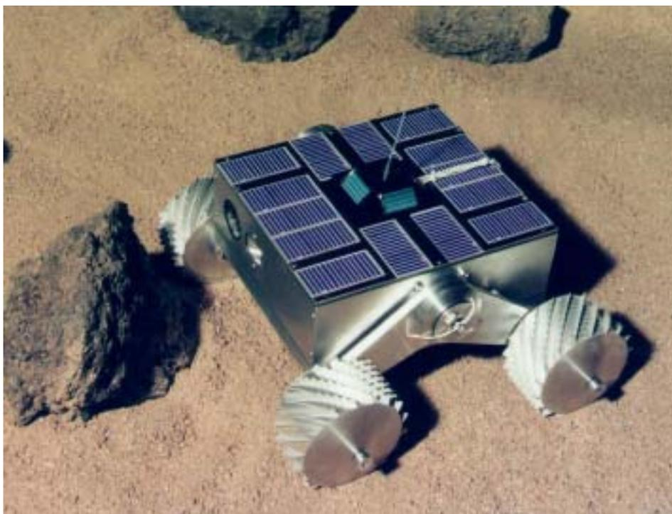
*Technological advances in intelligent robotics are an important step toward the in situ analytic capabilities on the surface of solar system bodies far from Earth. Developing robots, such as the “Nanorover” seen here, improves both government and commercial research efforts in the fields of nanotechnology and autonomous microrobotics. (Source: NASA/Jet Propulsion Laboratory-Caltech)*
