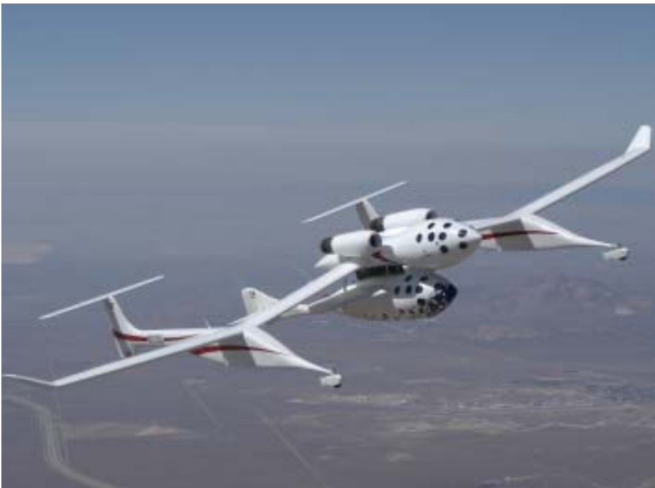
The White Knight turbojet aircraft climbs over the Mojave Desert with SpaceShipOne, the first private, piloted vehicle to reach an altitude of over one hundred kilometers. (Source: Scaled Composites, LLC)
