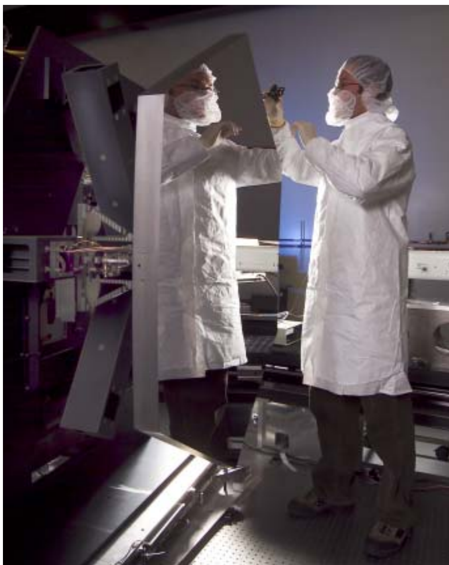
A technician mounts hardware on a mirror segment developed through a demonstration program for the James Webb Space Telescope. The telescope’s primary mirror will consist of eighteen hexagonal beryllium segments that will span 6.5 meters when the telescope begins operations. (Source: Northrop Grumman Space Technology)
