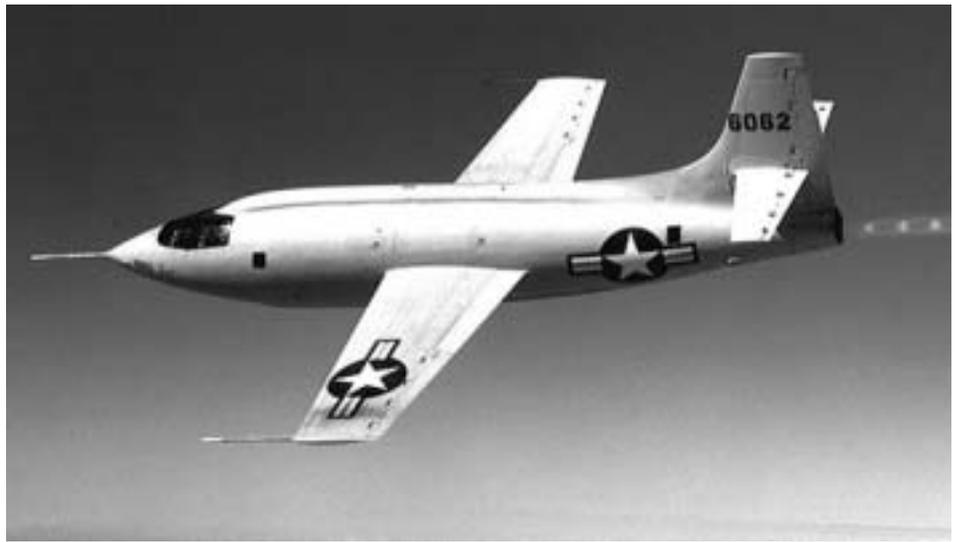
Made famous by Chuck Yeager's successful first flight through the sound barrier in 1947, the Bell X-1 rocket plane closely resembles *SpaceShipOne* in fuselage shape and its completely faired-in canopy. Besides *SpaceShipOne*, the X-1 is the only other supersonic vehicle to have employed manual flight controls. (Source: NASA)
