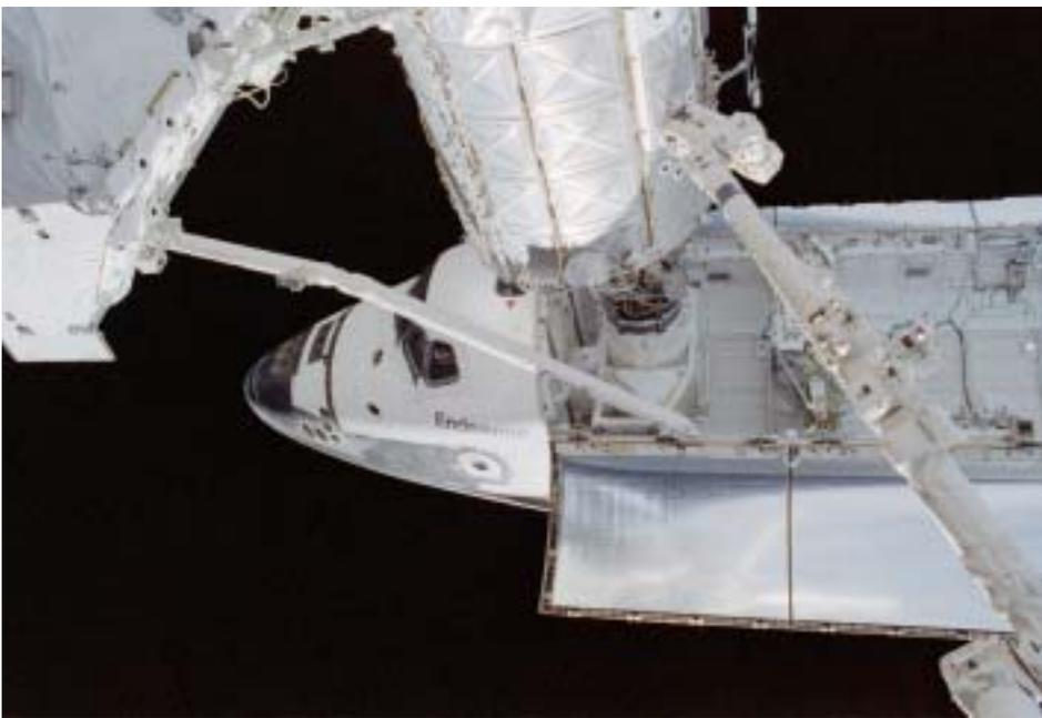
*The space shuttle was designed to be a remarkably versatile vehicle, outfitted with a sizable payload bay, a robotic manipulator arm, and the capacity to carry humans and heavy payloads to and from Earth orbit. (Source: NASA)*
