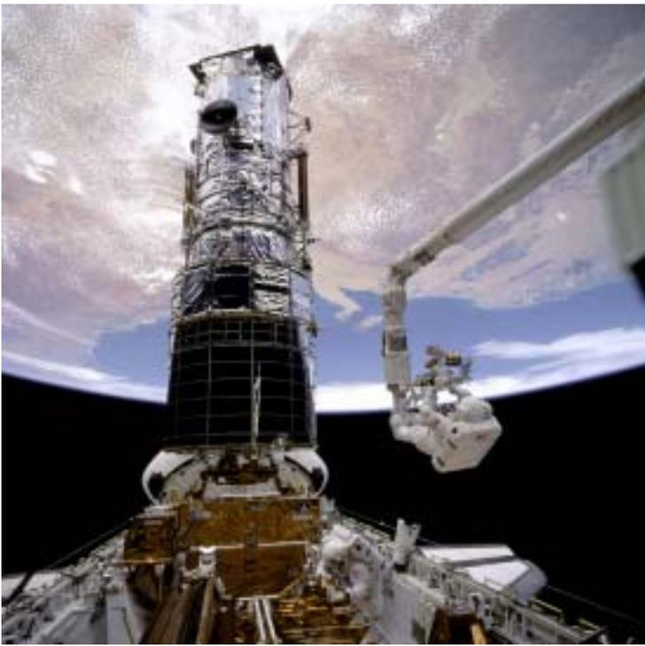
*Astronaut F. Story Musgrave, anchored on the end of the Remote Manipulator System arm, prepares to be elevated to the top of the Hubble Space Telescope to install protective covers on the magnetometers. Humans and robots have provided mutual support to one another in space exploration pursuits—and will continue to do so. (Source: NASA)*
