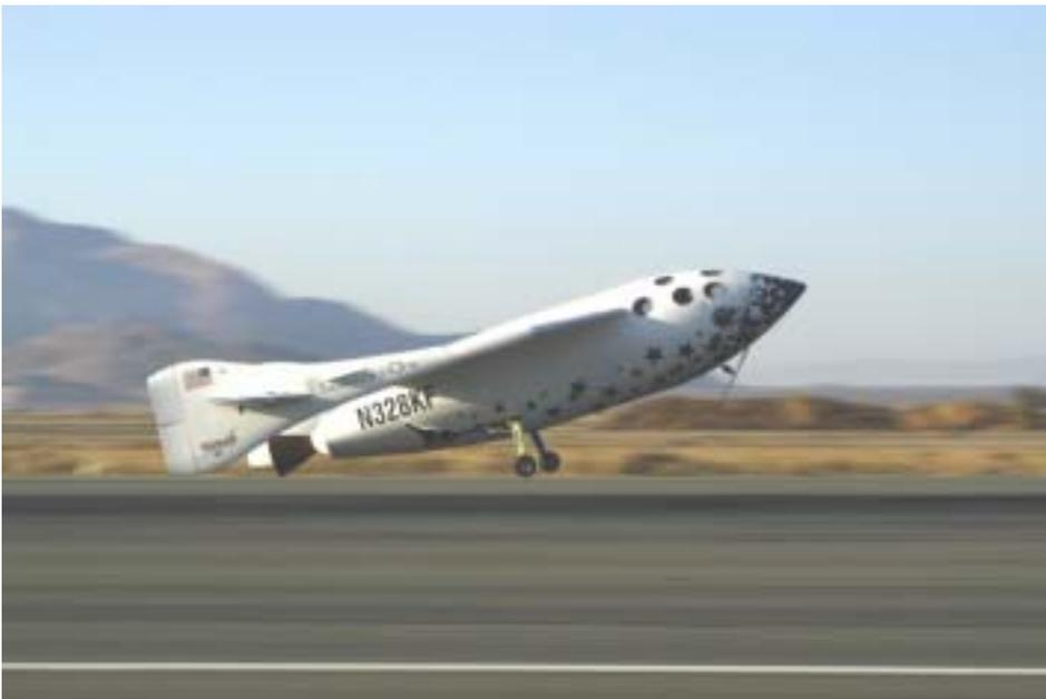
Having reached almost Mach 3 on its first flight to space, SpaceShipOne is engineered to control well at supersonic speeds, but the vehicle also functions as a good glider. Like craft such as the X-1, X-15, and the space shuttle orbiter, SpaceShipOne glides in for recovery and landing. Seen here on a test flight, SpaceShipOne has a relatively low landing speed of 145 kilometers per hour. (Source: Scaled Composites)
