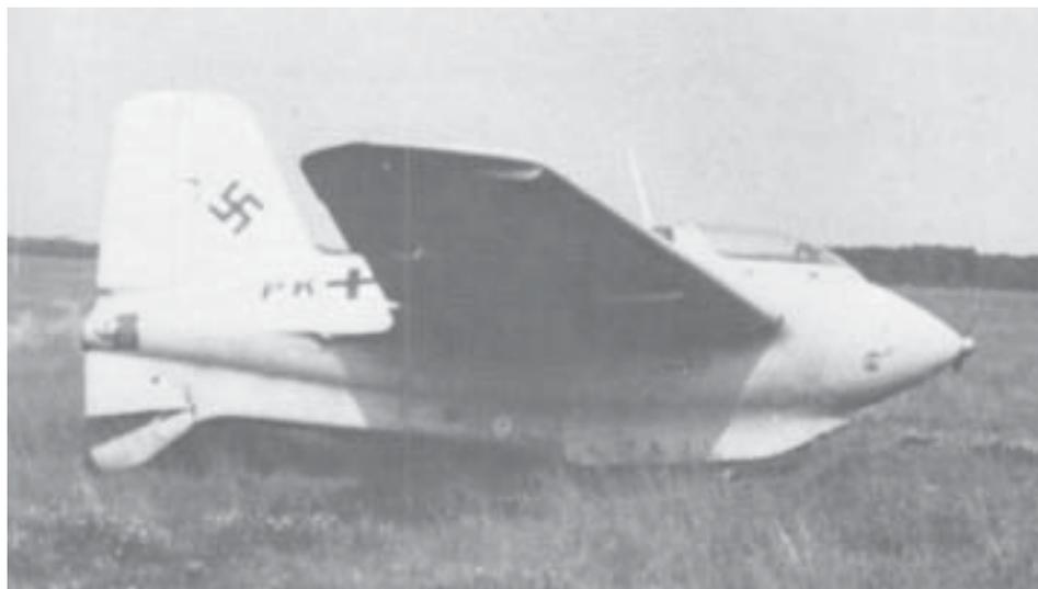
*The Messerschmitt Komet was a German rocket plane of World War II that pioneered spectacular velocities and climb rates: it could hit almost 970 kilometers per hour and climb 12,000 meters in three minutes. It was the only rocket interceptor ever fielded. Through "convergent evolution," Komet's fuselage profile very closely resembles the profile of SpaceShipOne. (Source: Jeffrey L. Ethell)*
