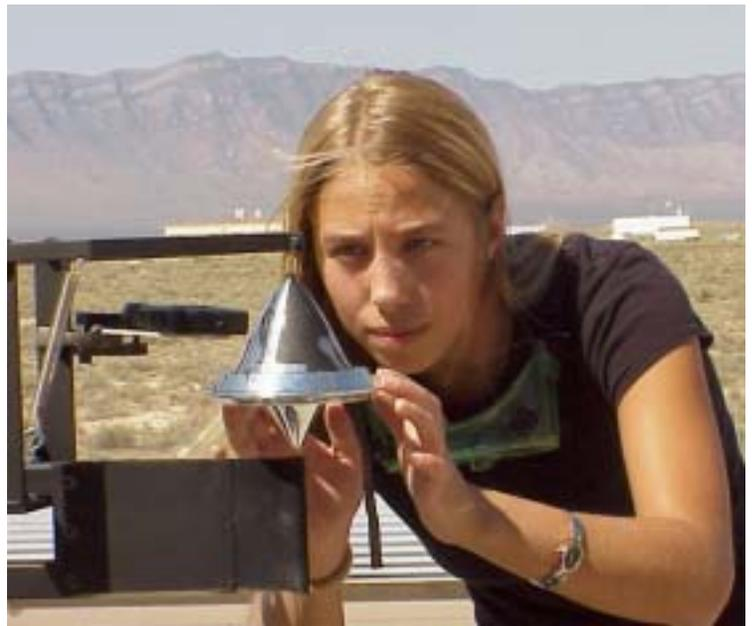
*Tregenna Myrabo of Lightcraft Technologies, Inc., prepares a laser-propelled lightcraft for launch at White Sands Missile Range in New Mexico. The lightcraft, weighing 50 grams and made of ceramic materials, was boosted by a laser beam to an altitude of seventy-one meters in October 2000. (Source: NASA)*
