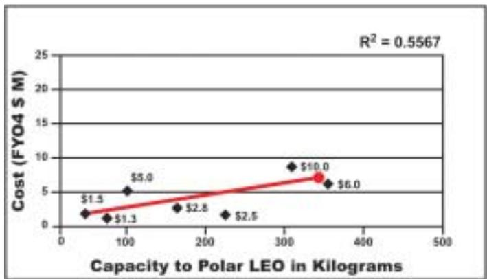
Figure 2: Weight versus cost (excluding flight-proven systems)
