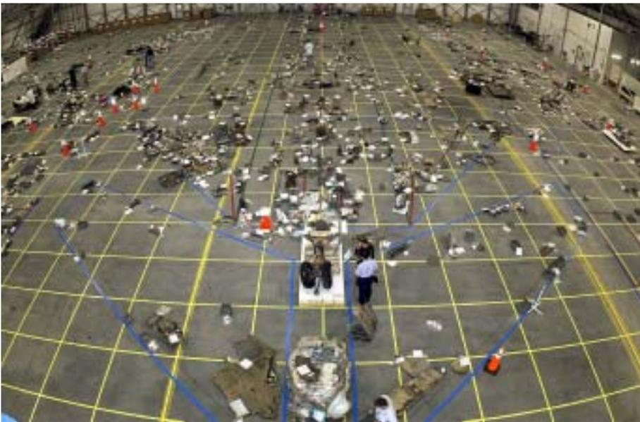
**ABOVE:** After the Columbia accident, investigators recovered debris and laid them out on a grid to show their location on the vehicle. They then studied the pieces to learn about the failure. (Source: NASA)
