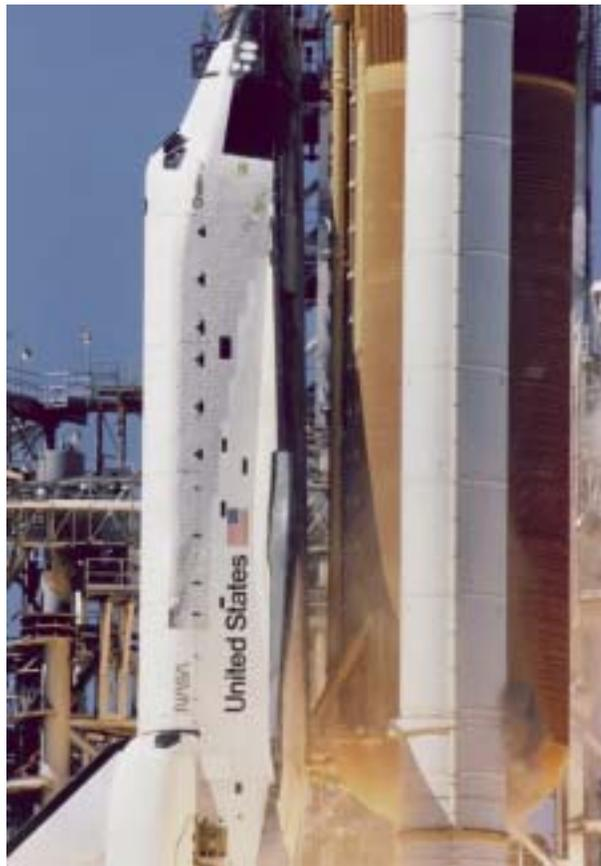
*Key evidence that a field joint on the right solid rocket motor had leaked before the Challenger incident was this image of a puff of gray smoke, seen in the lower right. (Source: NASA)*
