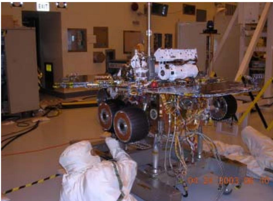
*Technicians swab small surfaces on one of the Mars Exploration Rovers in order to document any microorganisms that the spacecraft may carry with it to Mars. (Source: NASA/JPL)*
