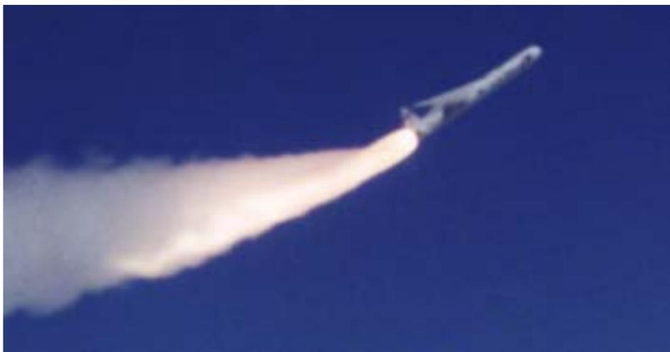
Pegasus small launch vehicle after release from launch aircraft. (Source: Orbital Sciences Corporation)
