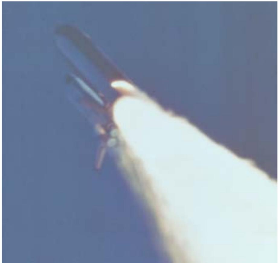
*The plume of flame from Challenger's right solid rocket booster indicated the failure of the field joint. (Source: NASA)*
